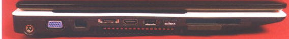
On this side of the laptop, we find the power-supply input, D-sub and HDMI outputs for a second monitor, an RJ45 port and two USB 2 ports, one of which is occupied by an Edimax Wi-Fi adaptor. Other connections are found on the back and at the other end of the laptop.
